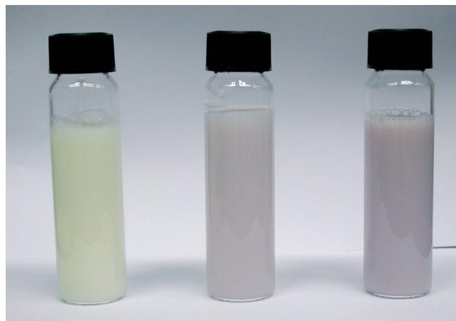
Figure 3. Photographs of aqueous solutions containing ceria nanocrystals with particle sizes of 3.5, 40, and 80 nm.
